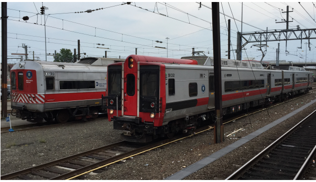
Figure 2: An M-2 (left) and M-8 (right) sit in the New Haven Yard.
