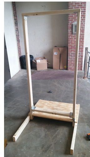
Figure 4: Image showing the fabricated support stand using construction lumber (pine). This stand would be used to hold the VAWT.
