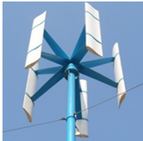
Figure 2: This is an example photo of a Vertical Axis Wind Turbine (VAWT).
