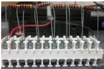
Figure 3: Depicts the series of resistors used to drop the peak voltage
